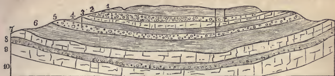
Fig. 91. Section from East to West across the lower peninsula of Michigan. 1, 2, 3, 4, 5, 6, etc. The several groups of strata from the Coal-measures to the Lower Silurian.
